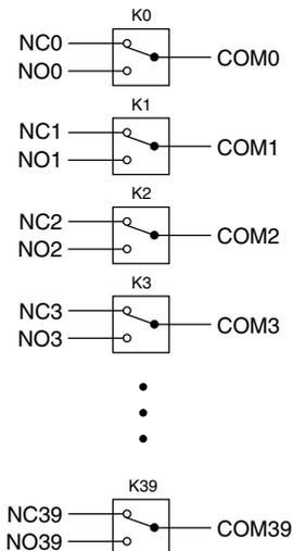
The following figure shows the PXI-2570 connector pinout.
